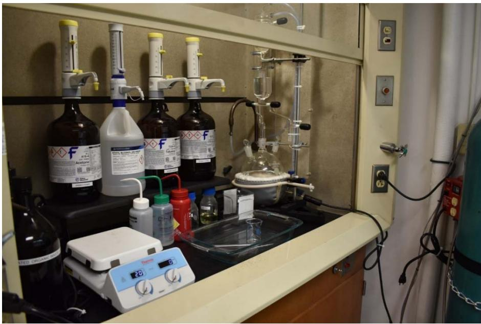
**Fume Hood:** The lab has a large fume hood that vents externally with a flow of over 900 Cubic Feet per minute.
